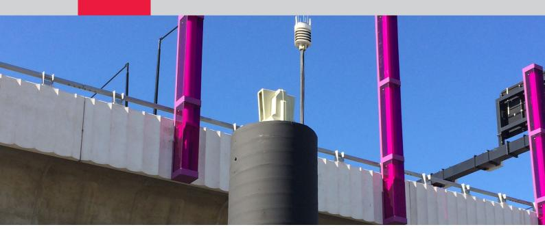
All of this combines to produce constant movement in a structure. Such movements are typically small and occur slowly over the cause of a day. It is critical, therefore, to understanding the structures' behaviour that monitoring is conducted automatically and frequently so that these changes can be tracked.
